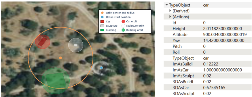
Fig. 7. Orbits and detected objects in GIS (left). Metadata of car GIS layer (right)
