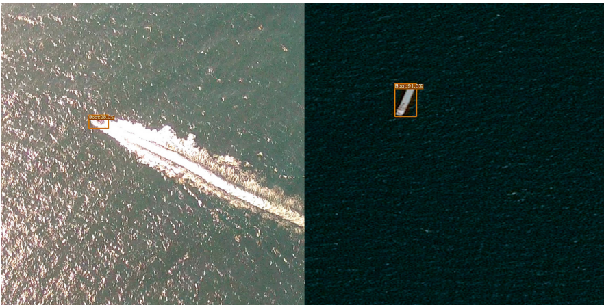
Fig. 6. Predicted labels on the Seagull and Airbus Ship Detection datasets using the SeaDronesSeeBoat model
